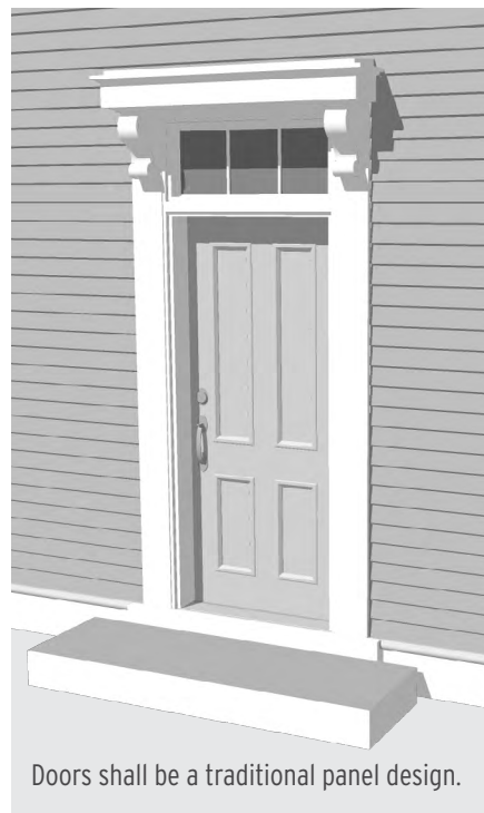
Figure 7.8 Door Design Requirements
