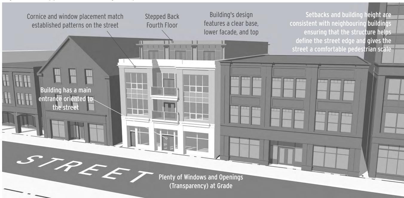
Figure 4.15: Applied Urban Design Requirements
