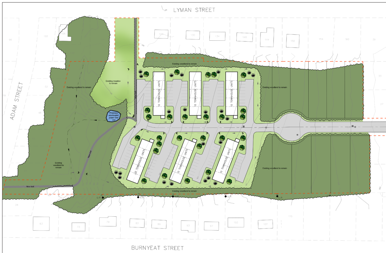
Site Plan submitted by Brentwood showing proposed configuration of six, one to two storey, 10 unit residential buildings
