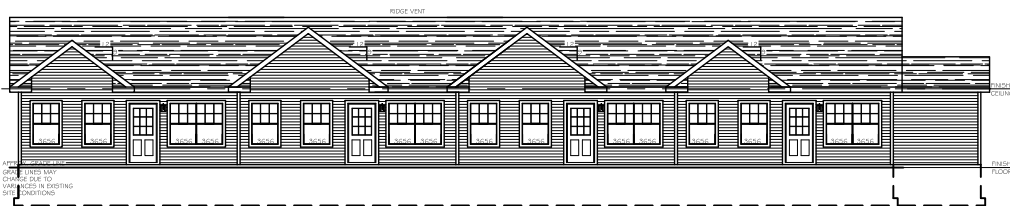
Front Elevation | one-storey 4-unit dwelling
