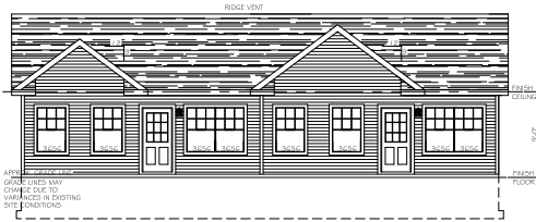
Front Elevation | one-storey 2-unit dwelling
