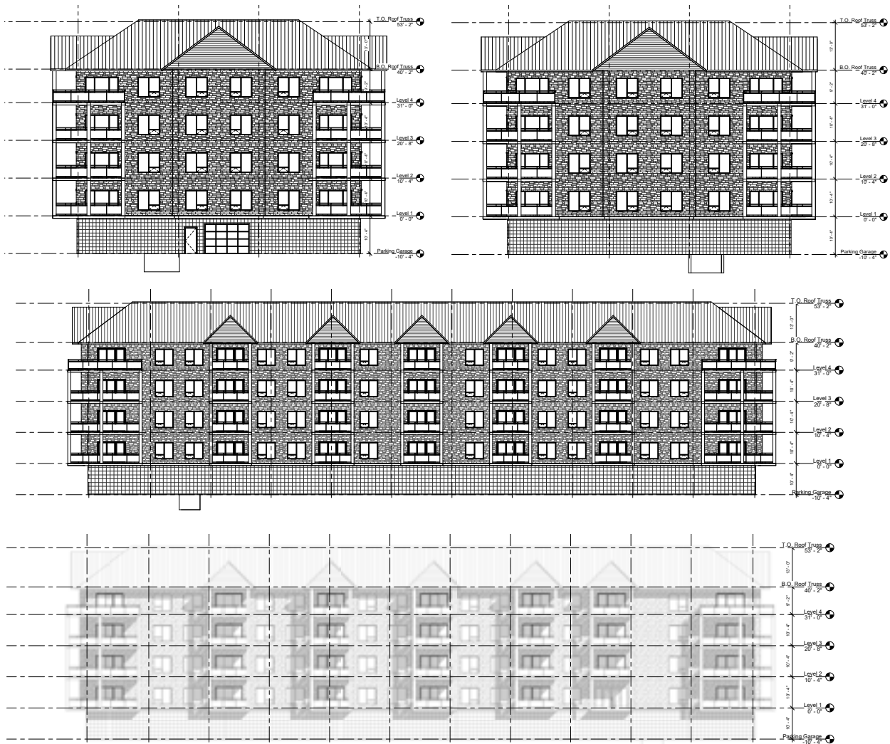
Typical Elevations of Proposed 50-unit Building
