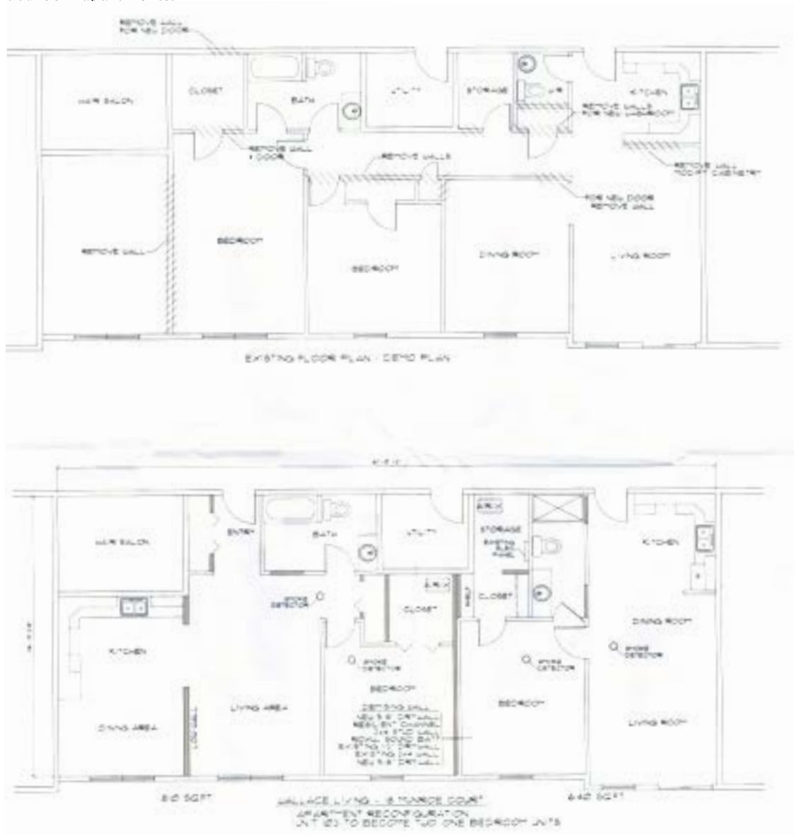
Floor Plan showing one of the existing 2-bedroom apartments and proposed two 1-bedroom apartments
